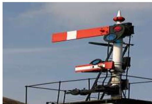
Trains cannot collide with each other if they are not permitted to occupy the same section of track at the same time, so railway lines are divided into sections known as *blocks*. In normal circumstances, only one train is permitted in each block at a time. This principle forms the basis of most railway safety systems
